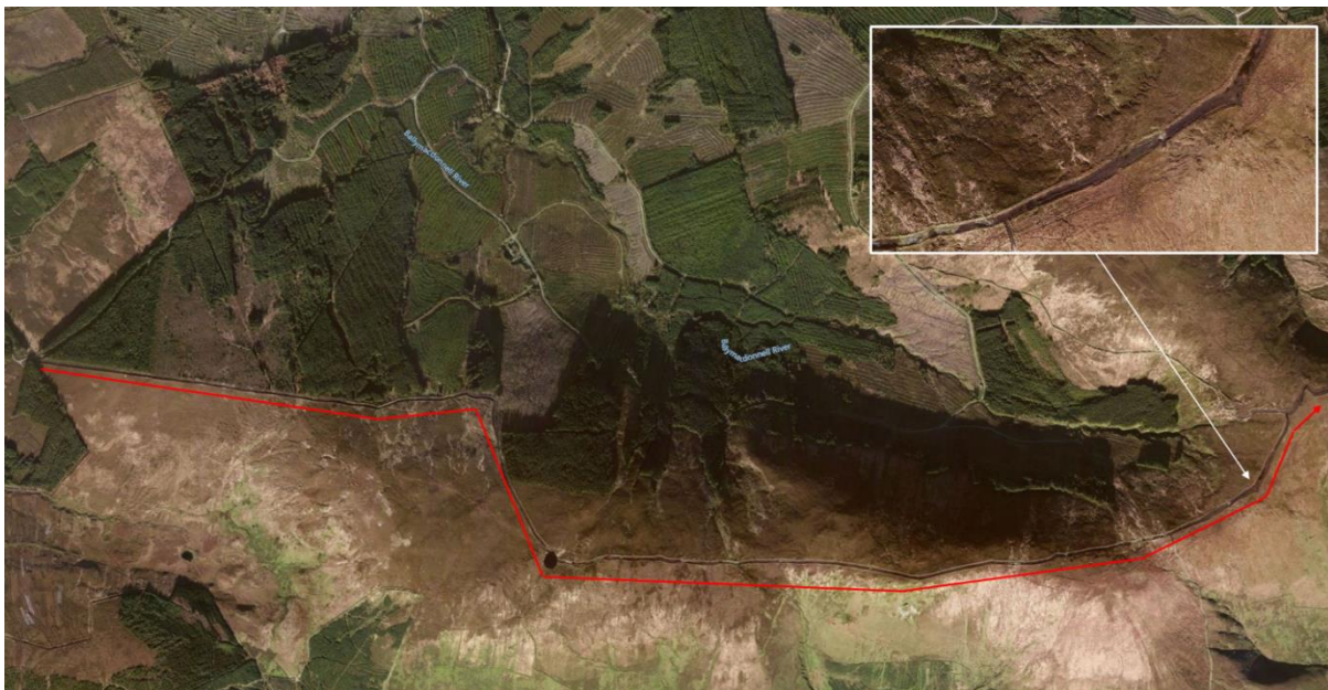
Figure 3-1 Significant fire break and hydrological break from peatland to the site.
